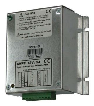
The units provide a "boost charge" input as a standard feature. When this input is pulled to battery negative, the output voltage of the charger will be set to the boost charge voltage. This feature may be used temporarily to improve battery life.
