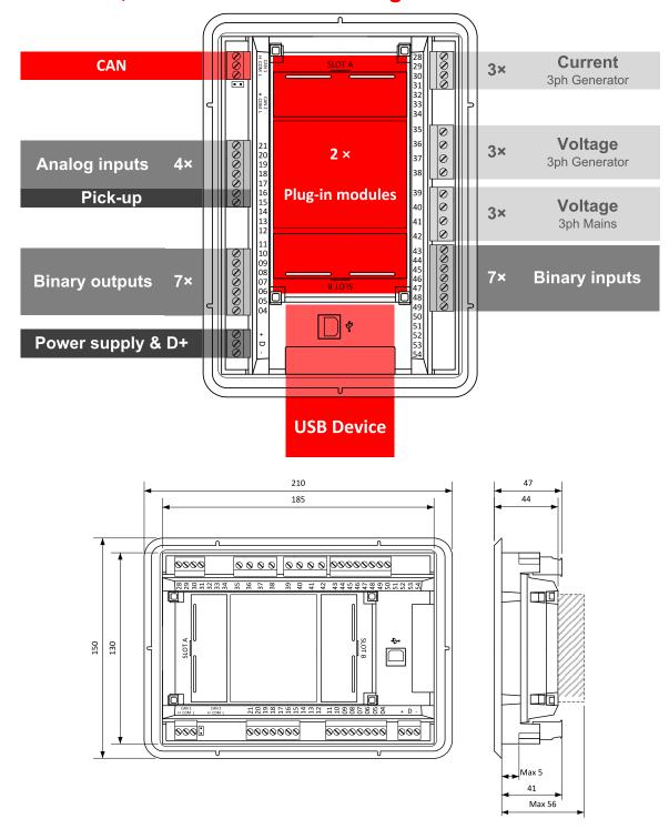
**Note:** The final depth of the controller depends on the selected plug-in module - it can vary between 41 mm and 56 mm. Mind also the size of connectors and cables (e.g. in case of RS232 connector, add about 60 mm more for standard RS232 connector and cable).
