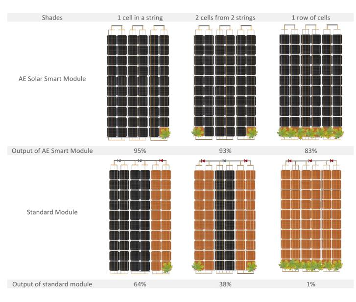
When multiple cells are in shade, a hot-spot free module can generate 80% more power, compared to a standard module.
